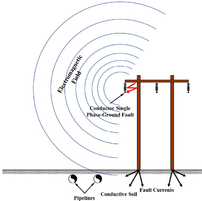
Figure 4. HVAC Fault Condition – Inductive and Conductive Interference
