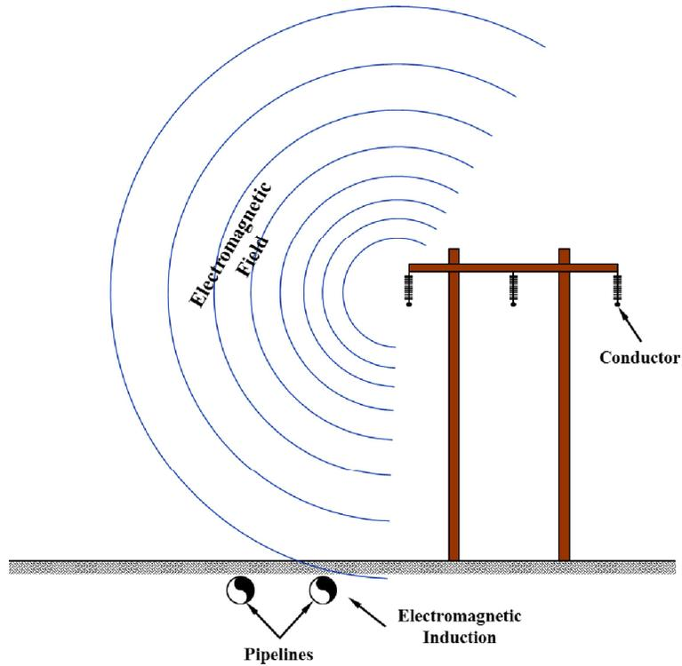
Figure 3. Steady State HVAC Interference – Electromagnetic Induction Effect
