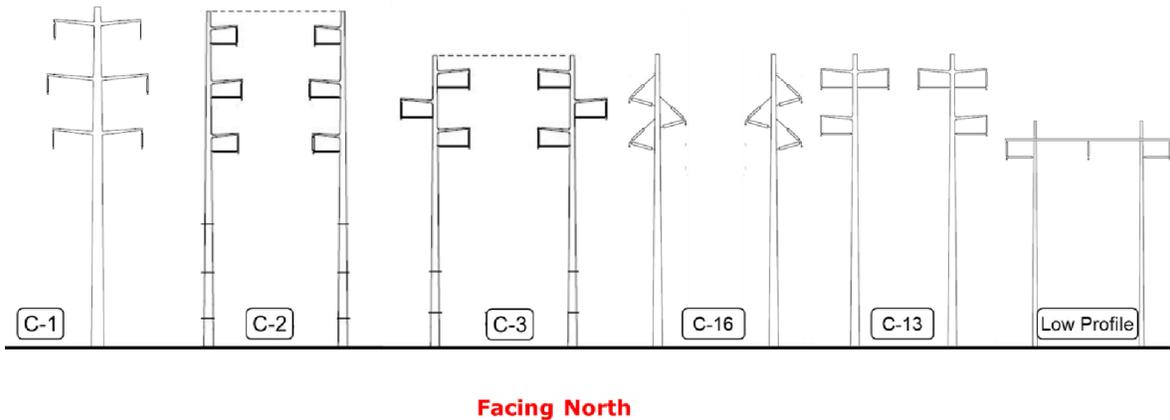
Figure 6. Pole Configurations Considered in the AC Analysis
